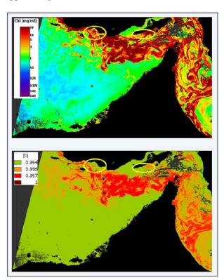
Figure 5. Chlorophyll map (top) ad HAB detection map (bottom) from a MERIS scene acquired the 30/12/2012. The HAB map was obtained applying three threshold values to the RI: red=high probability, green=no HAB. The yellow circles evidence different behaviours of the two parameters.
