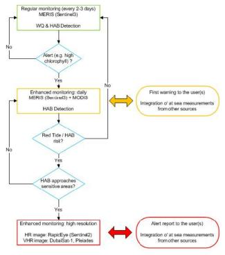
Figure 2. Flowchart describing the UAE Service Trial concept for HAB/Red Tide monitoring and alert
